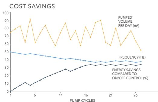
By finding the optimal frequency SmartRun will automatically reduce your energy bill up to 50%.
