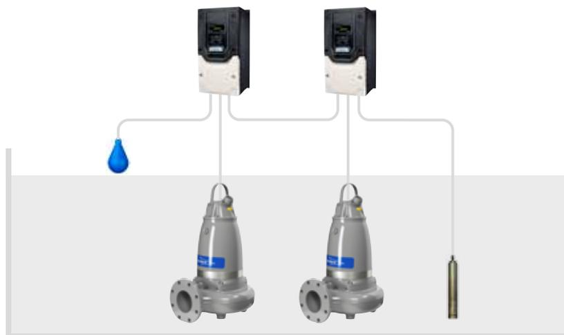
A SmartRun installation: two pumps, two SmartRuns, one level switch and one pressure sensor; a solution which provides redundancy.
