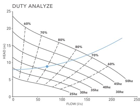
By constantly changing speed, SmartRun finds the most energy efficient frequency. In this way SmartRun avoids running at too low frequency, where energy consumption actually increases.
